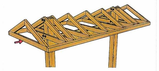
Attach the end roof joist structures to the fascia boards. Take care to ensure that the joist faces are vertical and flush with the fascia board and are plumb and true.
